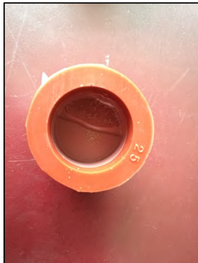
Epoxy embeds apatite grains slowly from one side. When the bottom of the form is filled slowly, fill about half of the form with epoxy. Avoid air bubbles. Photo: S. Falkowski.
