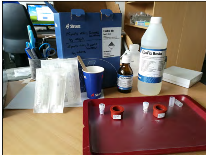
FlexiForms with interspersed grains ready for embedding and epoxy resin utensils. Photo: S. Falkowski.
