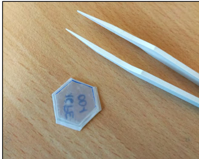
Package of apatite mount and mica external detector ready to be stacked with other mounts for irradiation. The sample ID is written on the back for easy handling (the sample ID is also scratched into the back of the mount but may be hard to read through the tape). Photo: S. Falkowski.
