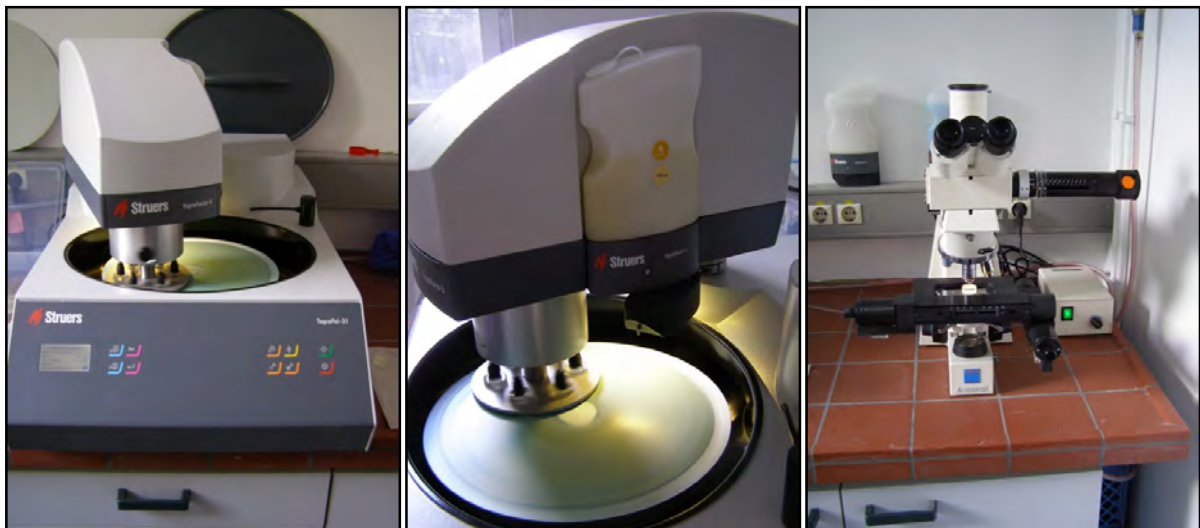
Left and middle: Polishing machine with sample holder for 6 mounts. The different pads for different polishing suspension sizes stick magnetically to the polishing wheel. The pads are kept in the drawers beneath the machine. Right: Microscope to check the polishing progress. Photos: E. Enkelmann.
