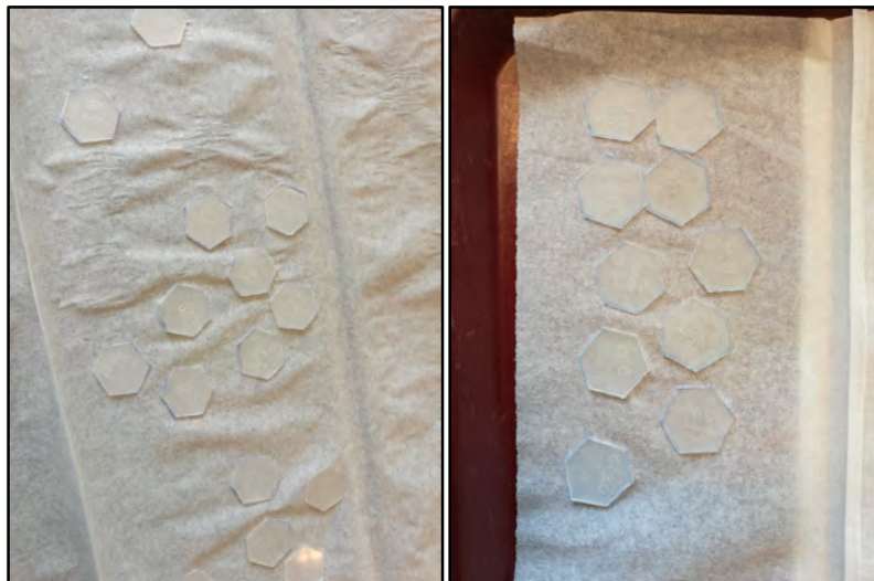
Apatite fission-track mounts after being cut into a hexagonal shape (20 mm diameter). The sample ID is scratched into the back of the mounts. Photos: S. Falkowski.
