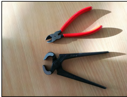
Pincers for bringing mounts from their round into a hexagonal shape. Photo: S. Falkowski.
