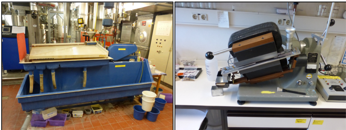
Left: Shaking water table for density separation. Right: Magnetic separation.
