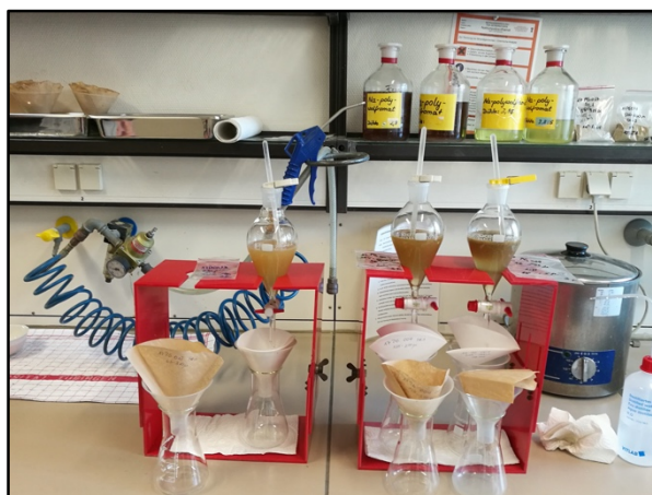
The density separation is carried out in two steps. First sodium polytungstate is used to separate minerals heavier and lighter than \sim 2.8 \text{ g/cm}^3 (picture). Then, diiodomethane with a density of 3.32 \text{ g/cm}^3 is used to separate apatites ( 3.2 \text{ g/cm}^3 ) and zircons ( 4.7 \text{ g/cm}^3 ).
