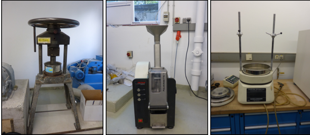
Rock crushing and sieving facilities: Press, jaw crusher, vibrating unit for up to seven sieves (left to right).
