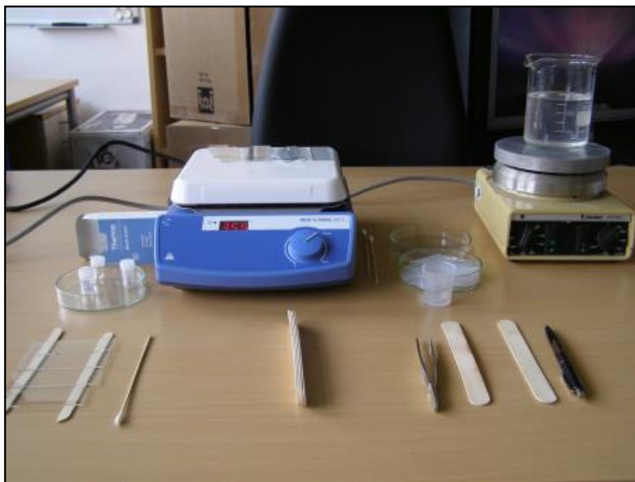
Zircon embedding utensils. Photo: E. Enkelmann.
