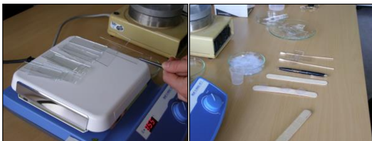
Left: The glass slides stick to the Teflon slide. Right: The glass slides and Teflon are placed on sticks to cool for a bit. Photos: E. Enkelmann.
