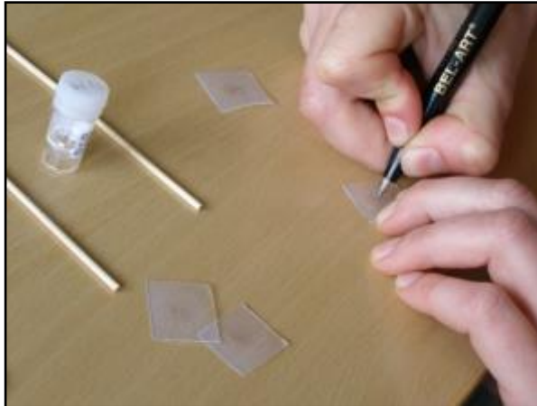
Scratching the sample ID into the back of the mount. Photo: E. Enkelmann.
