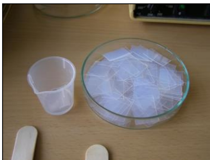
Cut Teflon slides and a small beaker with ethanol to wash Teflon before use. Photo: E. Enkelmann.
