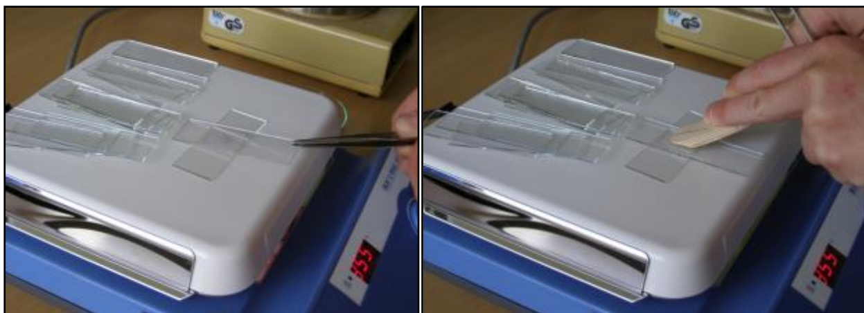
Right: A second, hot glass slide is placed on top of the Teflon slide in 90° angle to the first glass slide and then (left) pressed down on the Teflon slide with some wooden spatulas to embed the zircons in the Teflon. Photos: E. Enkelmann.
