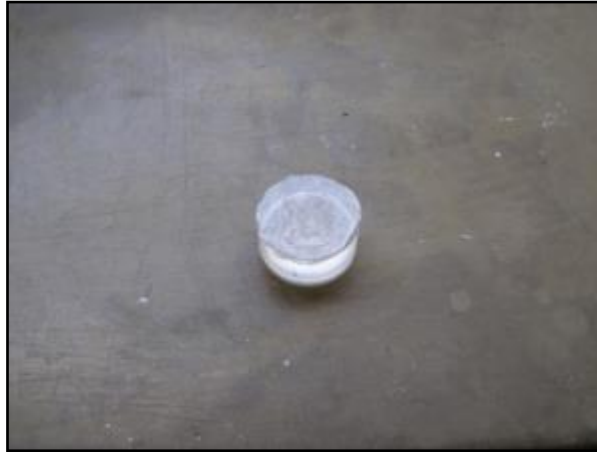
Epoxy dummy with double-sided tape and a Teflon ZFT mount. Photo: E. Enkelmann.
