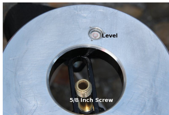
Figure 5: Interface Plate of the Leica Tripod with level and 5/8" screw.
