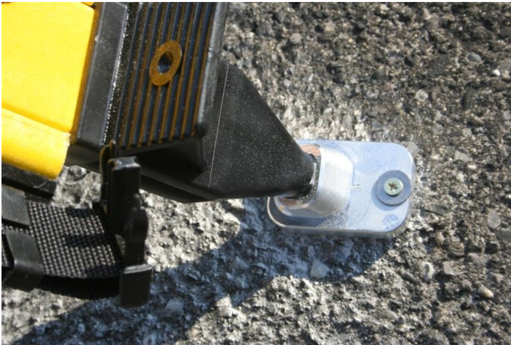
Figure 24: Tripod mounting adapter for screw anchor mounting.
